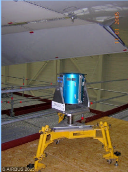
EX 520 C50 modal shakers used during the A380 GVT performed by the ONERA-DLR joint team (project leader ONERA) Pictures copyright AIRBUS S.A.S.
