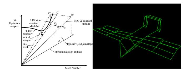
The results are presented as it is recommended in the Aviation Rules CS 25 (part AMC 25.629 – "Acceptable Means of Compliance"). These pictures are: frequencies vs. airspeed (or density), damping factors vs. airspeed (or density), critical velocity vs. Mach number and so on. Such pictures allow not only estimating flutter boundary, but also finding actual margins, necessary for the safety and certification. Flutter modes can be animated using standard P-Win-Modal option.
