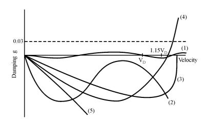
The solution of the typical flutter equation is performed in the subsonic and supersonic ranges by the **p-k** method for constant altitude (different max number) or constant Mach number (different altitudes). The only computational difference between these two cases is the way of computing the aerodynamic influence coefficients, using the **Doublet Lattice Method** in the subsonic range and the **Constant Pressure Panel Method** in the supersonic range.
